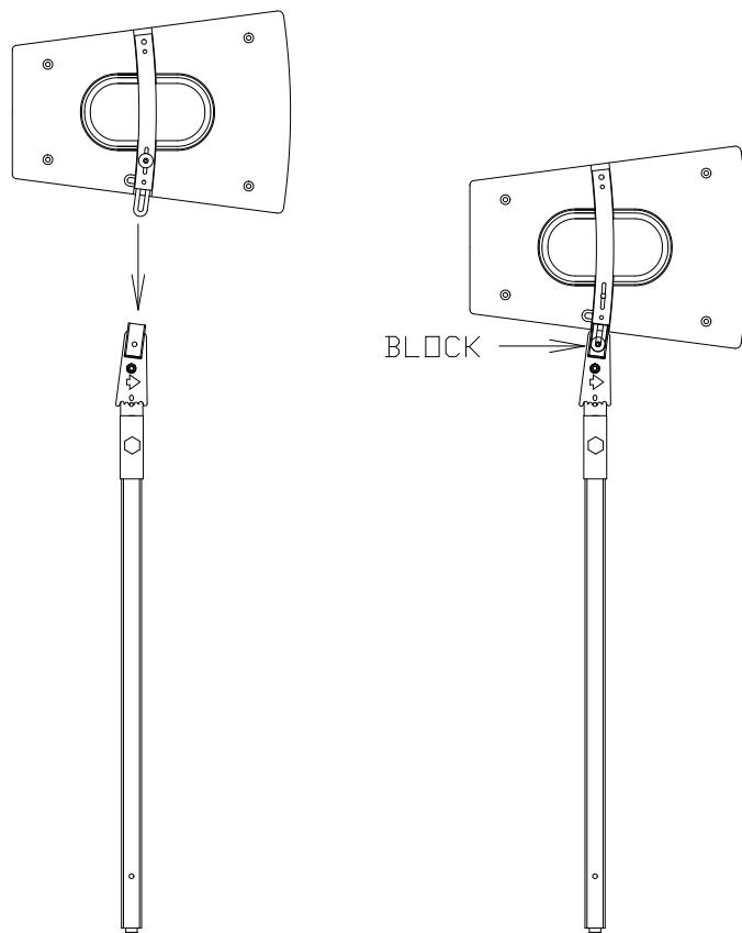
3- Tilt the cabinet as per the desired angle. To do so, just move upwards a little bit the box and block the desired position on the central metal guide.
