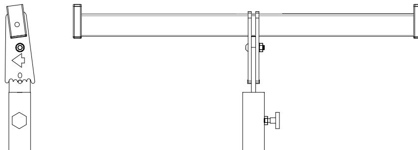
1- Place the PA-X12CL on top of a tripod or on top of the distance rod M20 bar. Once the PA-X12CL socket is received by the tripod or the distance rod bar, use the knob provided to attach both structures. Please, note that the arrow must be faceforward.
